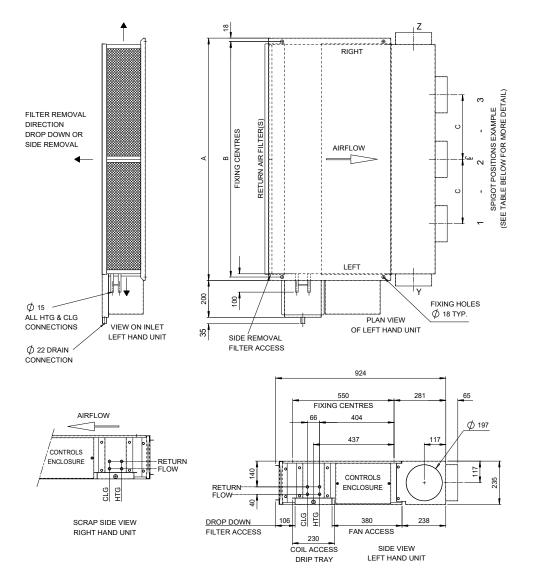
Units are handed looking against the direction of airflow, ie: looking into the discharge of the unit, with the unit in its installed orientation. General arrangement detail shows a fan coil with left hand coil connections.
